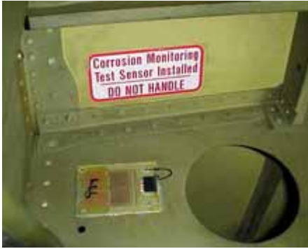
The cumulative environmental exposure sensor, pictured, is one of many that have been installed on the Air Force C-130 fleet. Photo courtesy of Air Force Corrosion Office.
