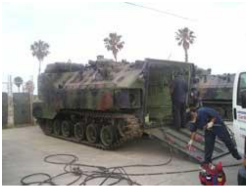
A corrosion service team member applies corrosion prevention compounds to the interior of an amphibious assault vehicle (AAV). Photo courtesy of the Marine Corps CPAC Office.
