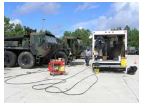
A corrosion service team member applies corrosion prevention compounds to a logistics vehicle system (LVS) at Marine Corps Base Camp Lejeune on the North Carolina coast. Marines use the LVS, nicknamed the "Dragon Wagon," to haul supplies from beachheads, ports, and airfields to combat service locations. Photo courtesy of the Marine Corps CPAC Office.
