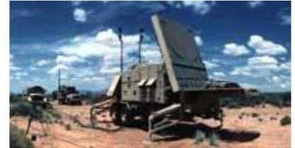
The Patriot radar set can detect, identify, classify, and track missile targets, as well as provide guidance and engagement support. AMCOM is taking steps to protect the radar system's vital cables from corrosion. Photo courtesy of AMCOM.
