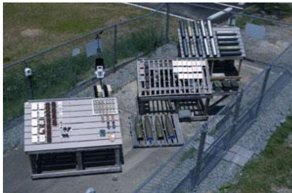
ARDEC offers a wide variety of corrosion test apparatus, such as the Corrosion Instrumented Test Yard (CITY). Photo courtesy of ARDEC.
